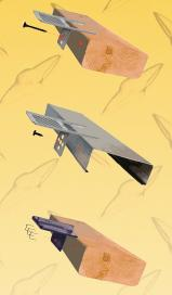
When fastening the HDPE plastic Nailer to a wood framing member use: two 1/2" staples (min.) with a 1/2" crown from an Arrow T-150 staple gun (or the like); one 1-1/4" drywall nail; or a 1" roofing nail.
